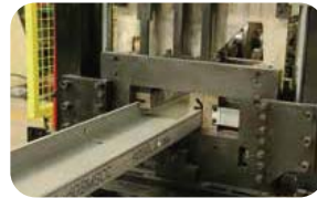
Patented Universal Post Cutter (With Patented Universal Post-cutter, Profile Forming More Stable)
